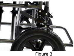
The user holds the brake handles with both hands when the wheelchair stops, and then moves the brake handles forward to self-locking condition, to make the rear wheels stop completely to keep still. The process for braking is completed. (Figure 3)
