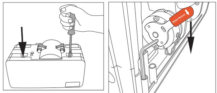
Push down and press cover outwards with a flat screwdriver in the two slots to open cover. Turn the "Brake Release" handle down. Locate sticker over the hole for manual emergency lowering. Punch hole or remove sticker and insert tool. Rotate counterclockwise to lower lifting belt. Using a power drill is recommended.
