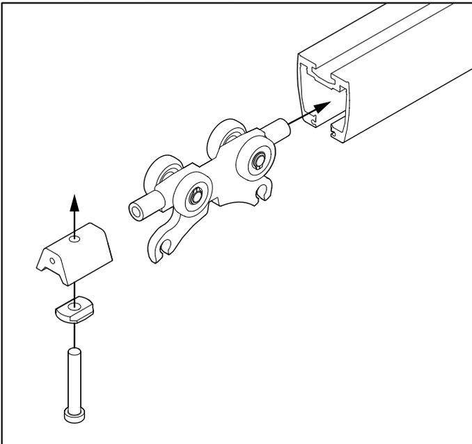
Remove End stop and insert Trolley into rail. Mount end stop, and make sure it is securely fastened
