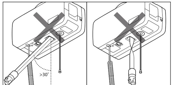
If the hoist doesn't respond to Hand control "up" button, it might be because lifting strap angle is too steep, or lifting belt is twisted and sensor is activated.
