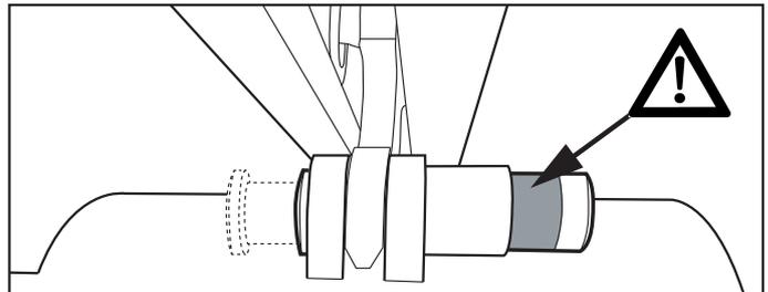
Make sure both connection point buttons completely return and clearly show green after installation.
