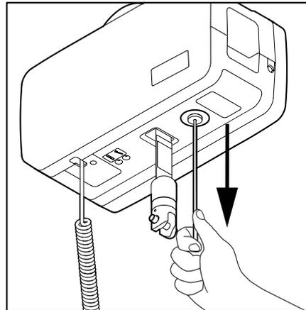
Pull and hold to start lowering. Hold until user is lowered and can be released from suspension.
