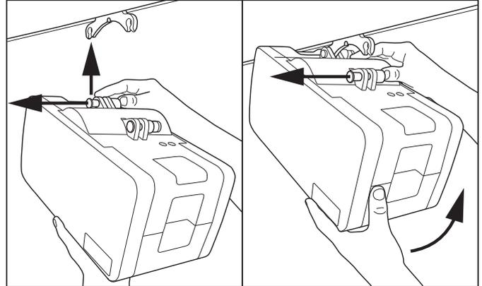
Connect one point first. Push button all the way in, and place lifter in connection point on trolley. Release button and make sure it is clearly showing green before connecting the next point.
