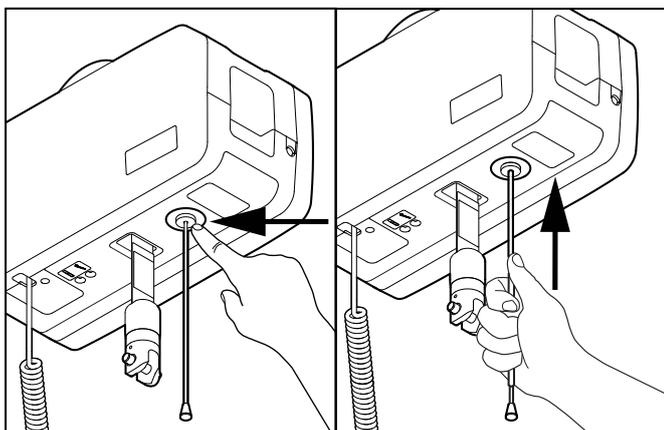
Push with finger or use tube on cord to push button back in to reset emergency stop.
