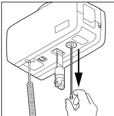
Pull to activate emergency stop. The button will come out, and hoist will stop.
