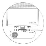
5. Peel off the Velcro fastener strip on the bottom of the wheelAIR® backrest cushion and feed through the top of the fan box.
