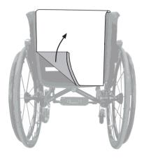
1. Remove the current backrest from your wheelchair, this should be easily removed from Velcro fastener strips beneath. Leave the suspension support structure attached to your wheelchair.
