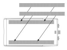
2. Determine whether your wheelchair support structure has hook or loop Velcro and add the loop Velcro strips to the wheelAIR® backrest cushion if necessary.
